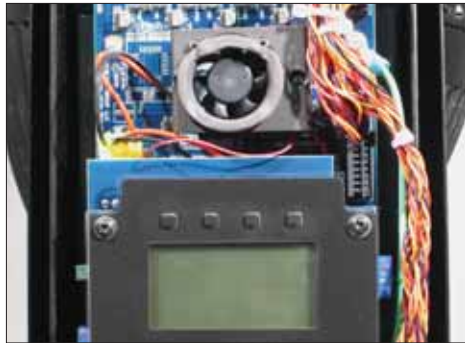
Fig 15. Motor control fan.
