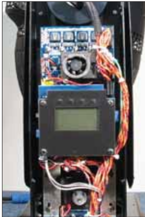
Fig 17. Motor control PCB and fan.
