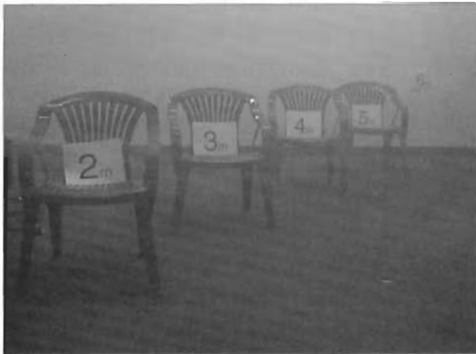
In this photo, fog density was 10mg/m 3 and general room lighting was used. Results with other densities were similar.
