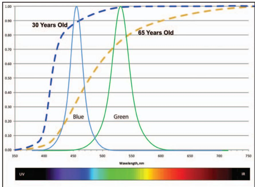
Figure 6 – Narrow band LED additive light source
