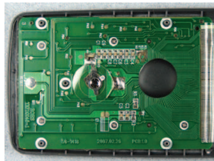
Figure 1 – Chip-on-board processor in a calculator
