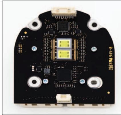
Figure 8 – Eviyos 2 Chip Layout
