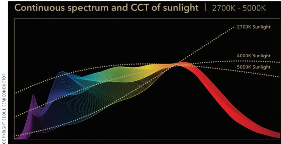
Figure 7 – SunLike phosphor mix options for varying color temperatures
