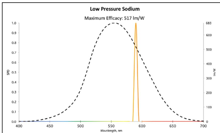
Figure 2 – Low pressure sodium
