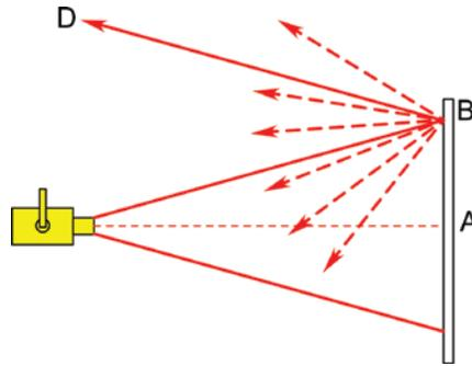
Figure 3 – Specular reflection
