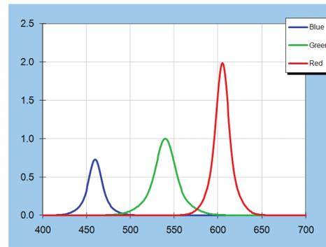
Figure 1 - Spectra of RGB LED with CRI of 81
