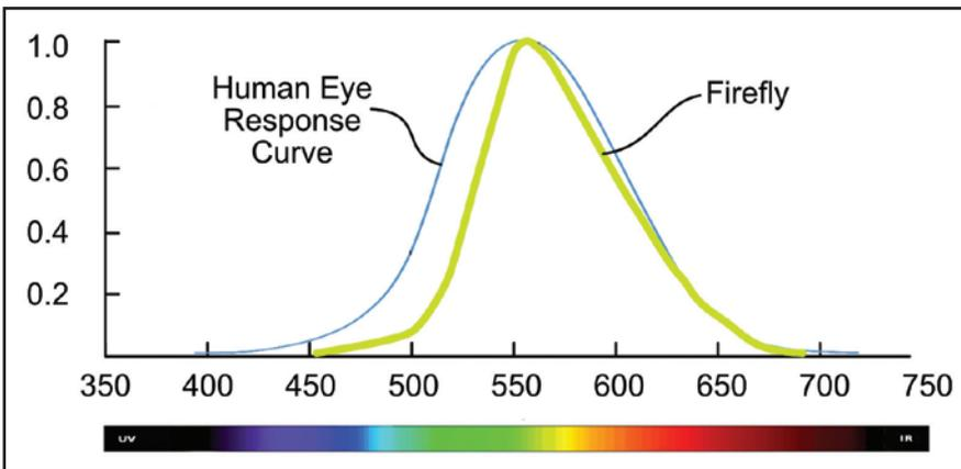
Figure 3 – Firefly spectrum compared with human eye sensitivity curve
