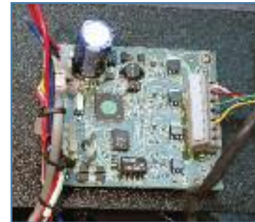
Fig 14 - Main control board
