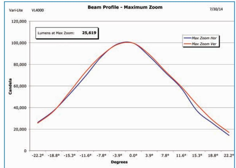
Fig. 16: Maximum beam profile.
