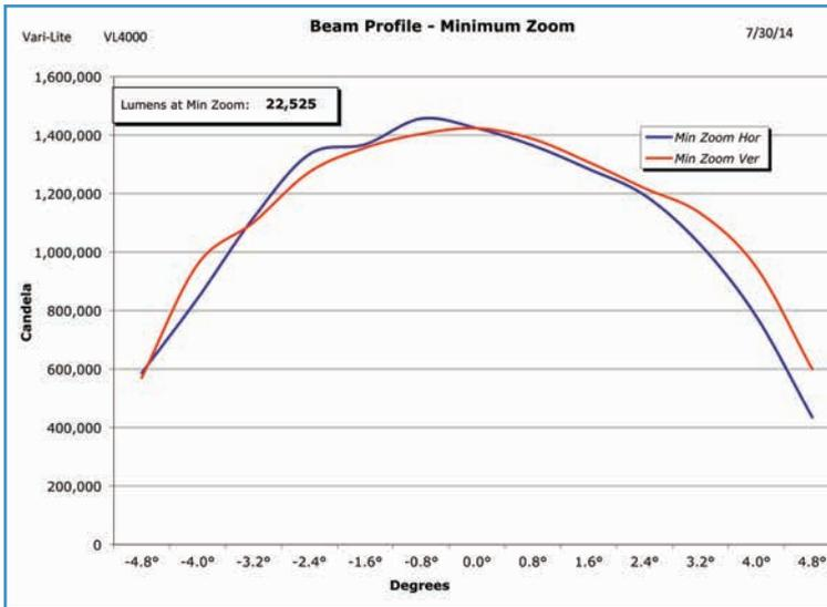
Fig. 15: Minimum beam profile.
