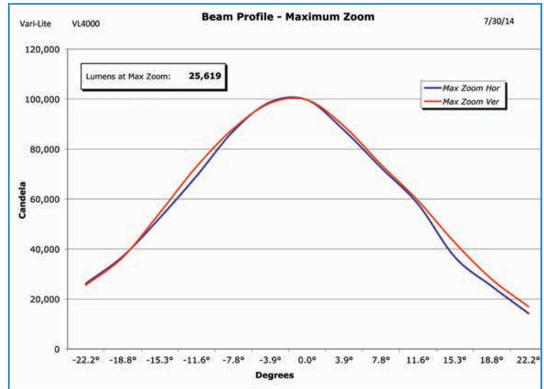
Fig. 16: Maximum beam profile.
