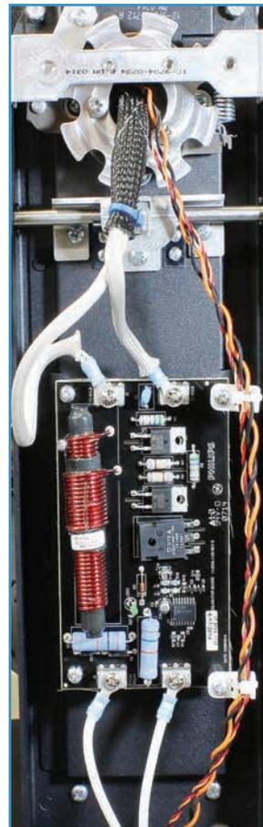
Fig. 20: Yoke with ignitor.
