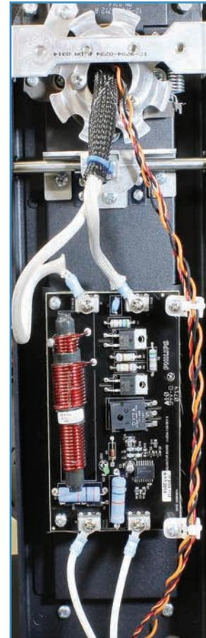
Fig. 20: Yoke with ignitor.
