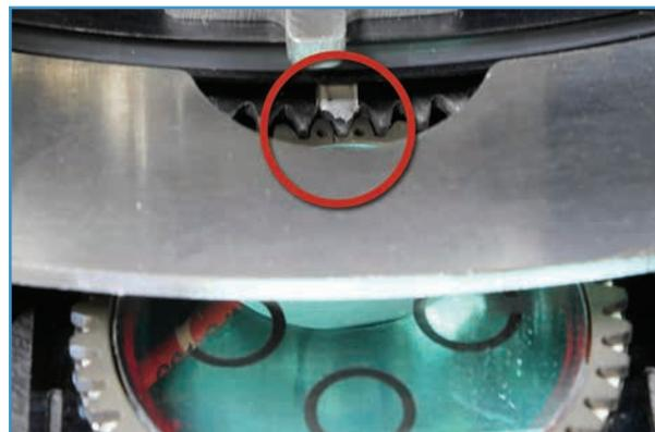
Figure 11: Gobo alignment marks.
