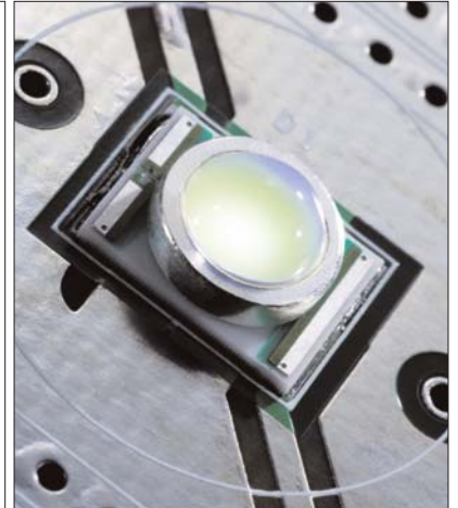
Figure 8: Cree XLamp, 75 lm/W white LED.
