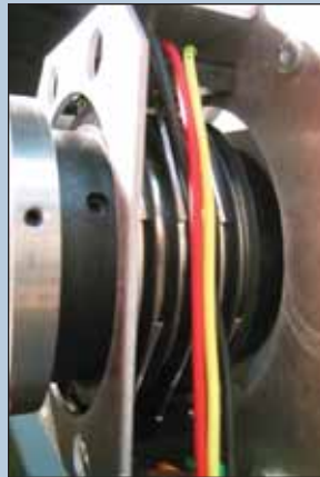
Fig. 19: Close-up of tilt slip ring assembly.
