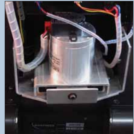
Fig. 20: Servo motor and encoder.
