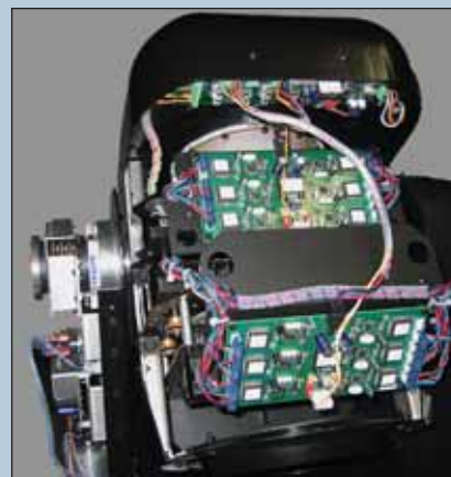
Fig. 4: Head showing removable modules.
