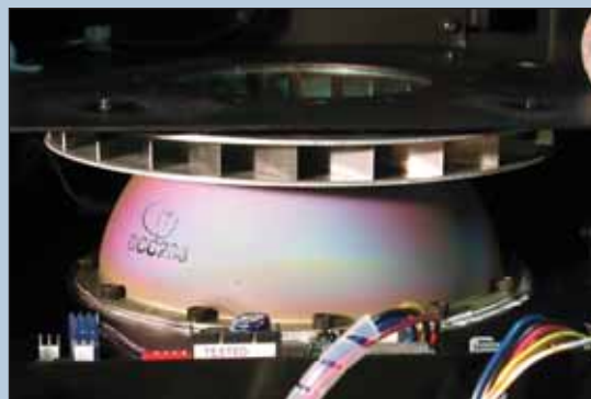
Left: Fig. 2: Lamp and connector. Above: Fig. 3: Reflector and cooling blades.
