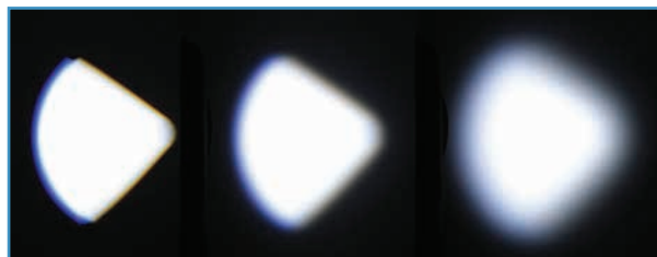
Figure 11: Framing and frost.
