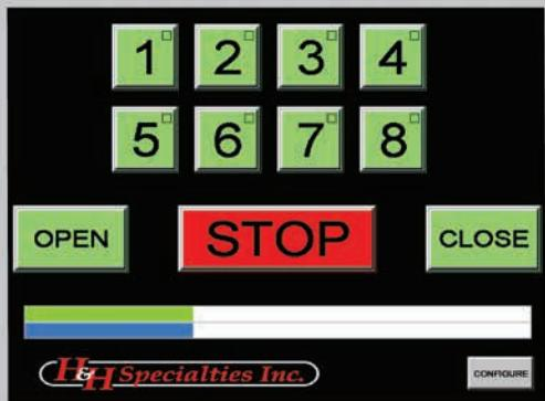
Programming the eight intermediate stops on the seven-inch touchscreen remote control is similar to an automobile radio.
