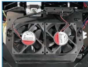
Fig. 3: LED module cooling.
