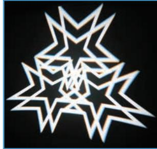
Fig. 11: Prism separation.
