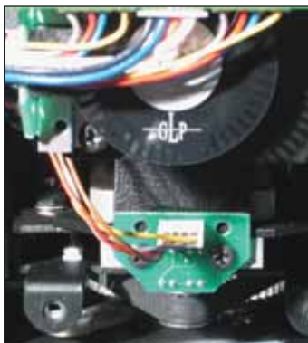
Fig. 9: Tilt encoder and pan gear
