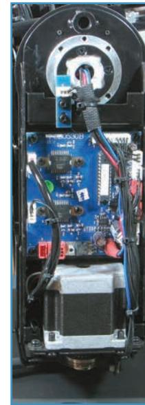
Figure 12 shows one yoke arm, which contains the pan motor and associated electronics. You can also glimpse the encoder wheel for the position feedback at the bottom of the photo. The other yoke arm contains the tilt motor. Finally, the top box contains all power supplies, as well as the menu and main control electronics (Figure 14). The Platinum Beam 15R Pro head is fairly cramped and not
