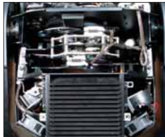
Fig. 5: Lamp house and optical assembly
