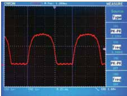
Fig. 10: Measuring strobe rate
