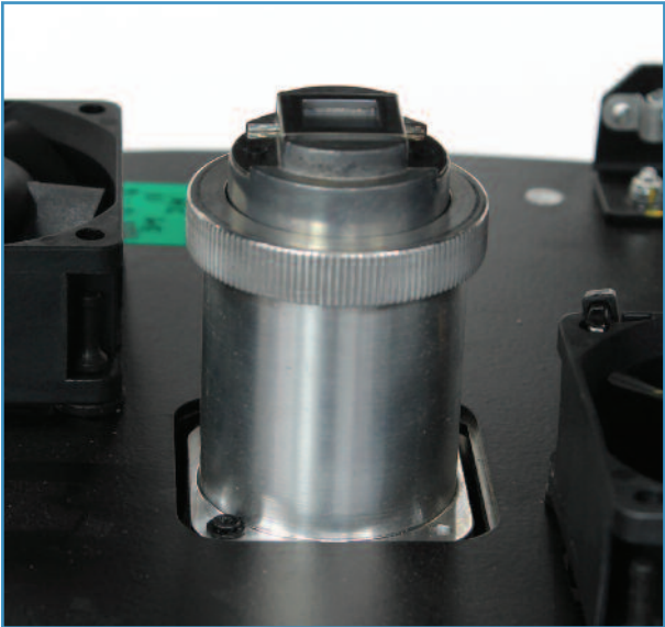
Figure 3: Light engine exit aperture.
