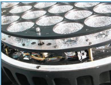
Fig. 6: Lens plate and actuator
