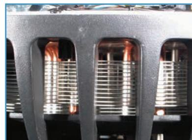
Fig. 3: Heat pipes and heat sink plates
