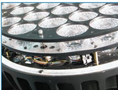
Fig. 6: Lens plate and actuator
