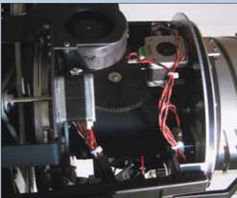
Fig 09: Caption: Focus lens assembly.
