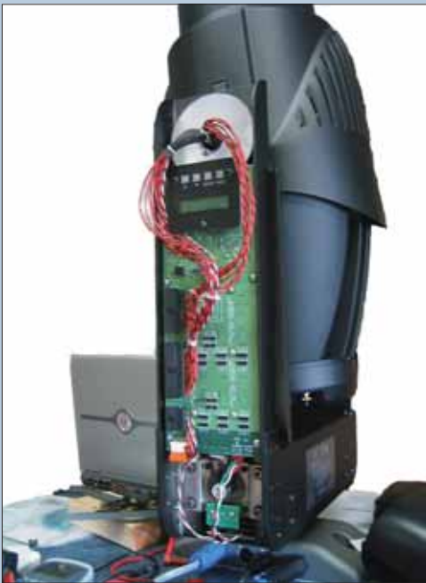
Fig 19: Side view of fixture showing electronics and tilt motor.
