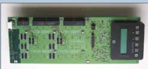
Fig 21: LCD display and control panel.
