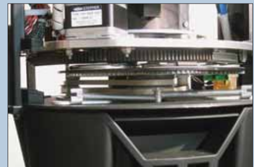
Fig 03: Gobo mechanism and driving belts.
