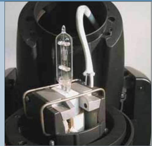
Fig 02: Lamp holder showing retaining clips and heatsinks.
