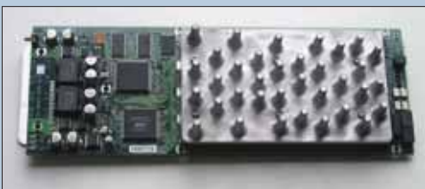
Fig 20: Heat sink behind motor control board, the tilt belt runs between the pins on the heat sink.
