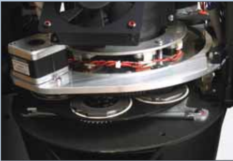
Fig 06: Caption: Gobo and framing shutter mechanism, note the thin framing module.
