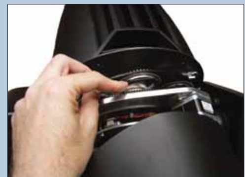
Fig 05: Gobo change, care needs to be taken to avoid scratching glass gobos on the retaining clip.
