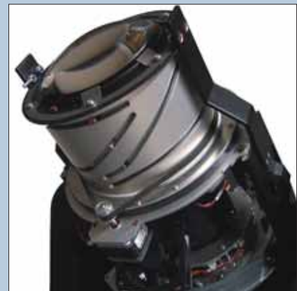
Fig 15: Zoom lens showing two cam slots for moving elements.
