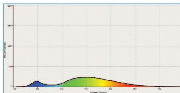
Figure 7: Spectrum - array white
