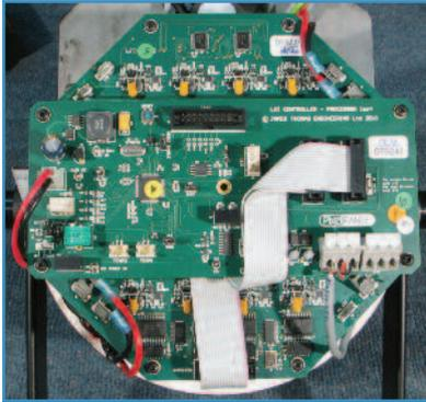
Figure 14: Control and LED driver boards
