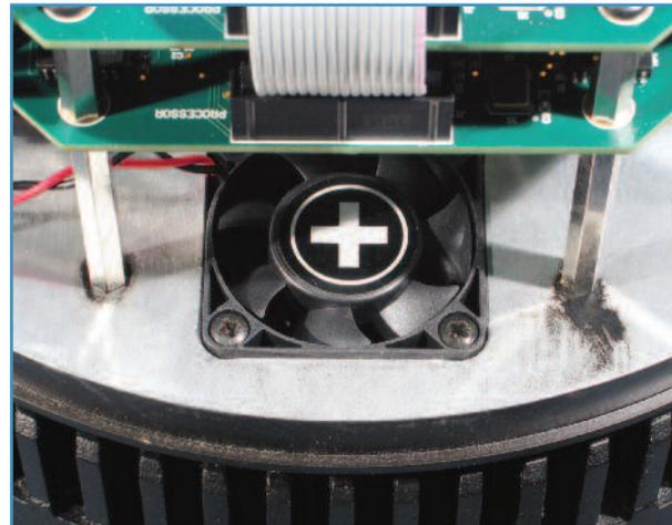
Figure 16: Heat sink fan
