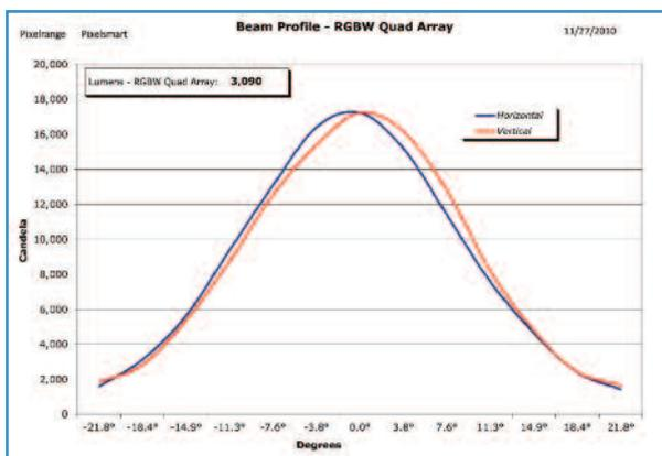
Figure 4: Output from RGBW array
