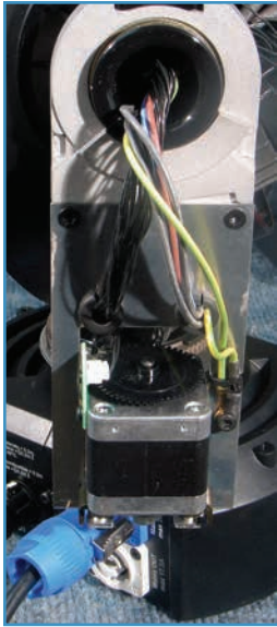
Figure 14: Pan motor and encoder
