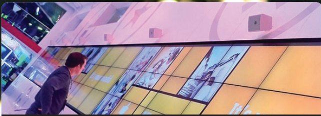
CES 2012: WATCHOUT orchestrates a 60 ft video wall with 63 screens. Image courtesy Mind Opera.
