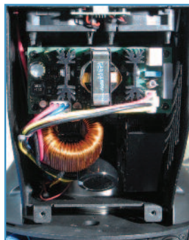
Figure 20: Power supplies in yoke
